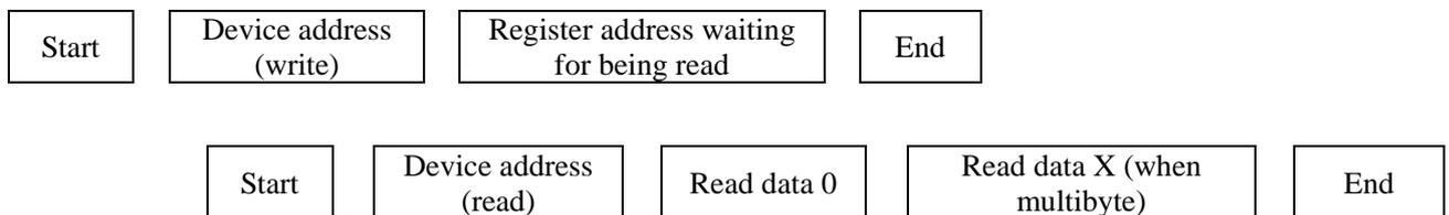
First use the device address of write to write register address waiting for being read, and then use the device address of read to read corresponding data.
